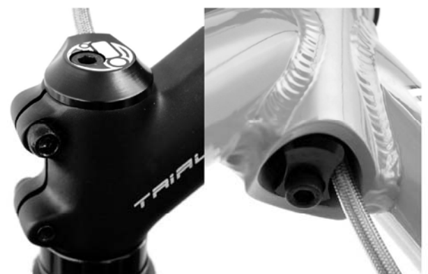
Fig.3 - Top Hose Enters On Non-Drive Side, Fit Bottom Bolt Towards Back.
