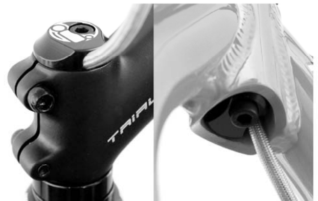
Fig.2 - Top Hose Enters On Drive Side, Fit Bottom Bolt Towards Front.
